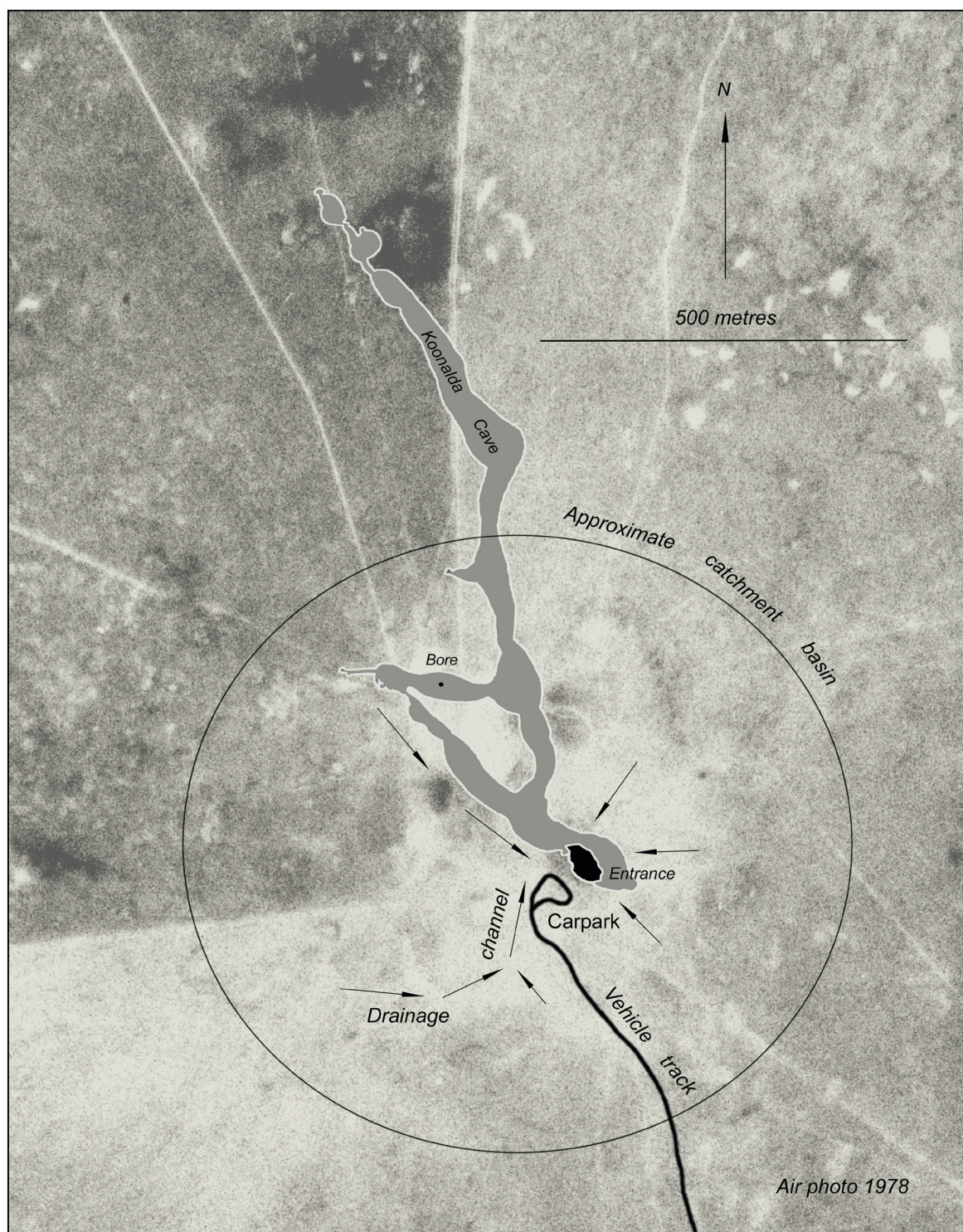
Figure 9. Koonalda Cave showing extent of surveyed passages in relation to selected surface features, including drainage channels, catchment basin (approximate), vehicle track and carpark. Other vehicle tracks not shown. Air photo 1978.
